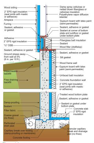
**Figure 14** Additional interior basement insulation
