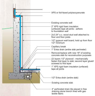
**Figure 15**Basement insulation with subfloor drainage
